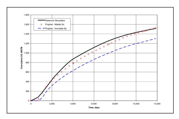
Similar *CO2-PROPHET* and full-scale simulator comparisons were completed for three additional oil fields - - Seminole (San Andres Unit), Wasson (Bennett Ranch Unit), and Vacuum (San Andres/Grayburg) (**Figures 8, 9** and **10**) - - again showing an excellent match between the two models when the oil saturation modification (discussed above) was included in the *CO2-PROPHET* input data set.
