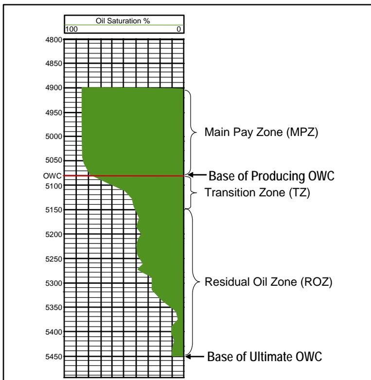
**D. Origin of Residual Oil Zones.** A number of possible actions may create a ROZ after the initial accumulation of oil in a reservoir. Specifically, the original oil accumulation may subsequently be affected by natural forces such as regional basin uplift, seal breach, or a change in the hydrodynamics of the underlying regional aquifer, leading to the development of an ROZ. Additional discussion of the origins and nature of ROZs is provided into previously prepared reports.<sup>5,6</sup>
