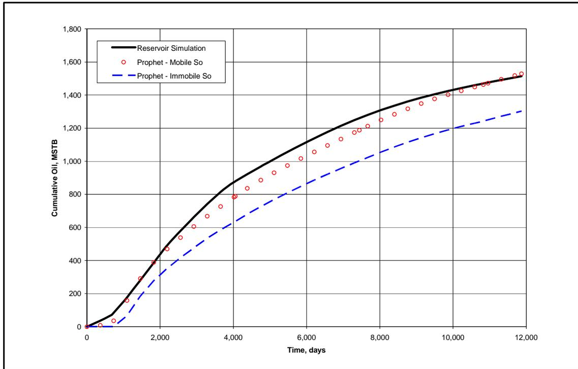
Similar *CO2-PROPHET* and full-scale simulator comparisons were completed for three additional oil fields - - Seminole (San Andres Unit), Wasson (Bennett Ranch Unit), and Vacuum (San Andres/Grayburg) (**Figures 7, 8 and 9**) - - again showing an excellent match between the two models when the oil saturation modification (discussed above) was included in the *CO2-PROPHET* input data set.
