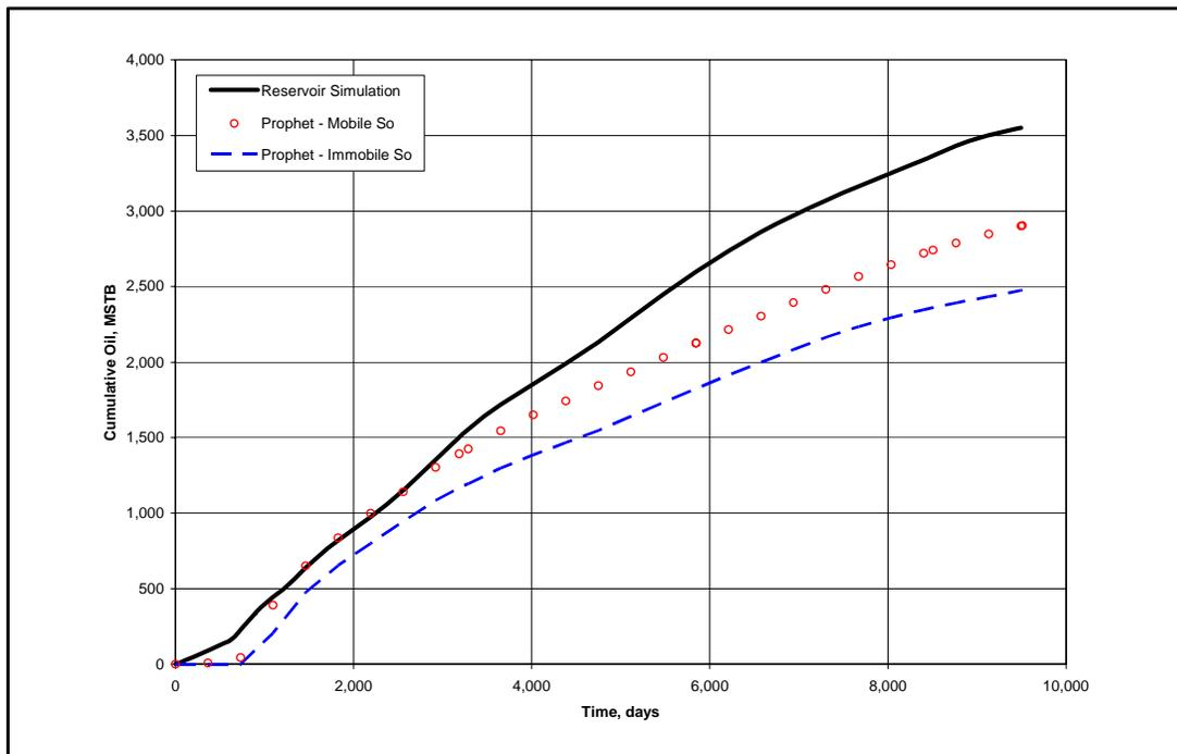
**Figure 8. Analysis of Simultaneous MPZ and TZ/ROZ Oil Recovery: Simulation Comparison Results, Wasson Bennett Ranch Unit**
